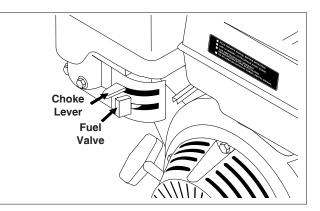
**STEP 6:** Rotate the fuel shut-off valve to the "On" position (fully counterclockwise on Briggs engines). Slide the fuel valve lever to the "ON" position (Honda engines). When the engine is not in use, leave the fuel valve in the "OFF" position.
