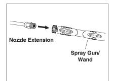
**STEP 2:** Attach nozzle extension to spray gun/wand. Tighten both by hand.
