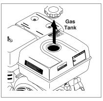
**STEP 3:** Fill gas tank with unleaded gasoline. Do not use leaded gasoline.
