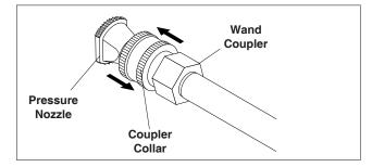
**STEP 7:** Pull the spring-loaded collar of the wand coupler back to insert your choice of pressure nozzle. Release the coupler collar and push the nozzle until the collar clicks. Pull the nozzle to make sure it is seated properly.
