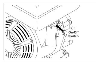
**STEP 8:** On Honda engines, turn the engine switch to "On" position.
