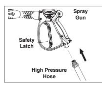
**STEP 1:** Attach the high pressure hose to the spray gun using teflon tape on hose threads.
