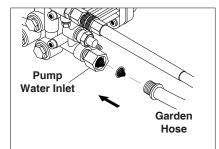
**STEP 5:** Connect the garden hose to pump water inlet. Inspect inlets. *CAUTION: Do not run the pump without water or pump damage will result.*
