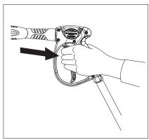
**STEP 5:** Trigger the spray gun to eliminate trapped air then wait for a steady flow of water to emerge from the spray wand. Then install nozzle.
