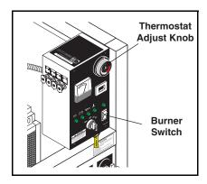
**STEP 4:** For hot water, turn the thermostat knob to 210° then push the burner switch to ON when a steady stream of water flows out of the spray gun. Burner will now light automatically. **NOTE:** Do not start machine with burner switch on.
