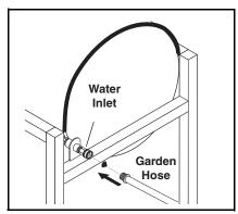
**STEP 1:** Attach a 5/8" water supply hose to inlet connector. Minimum flow should be 10 GPM depending on model of machine.
