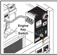
STEP 2: With the engine running, pull trigger to operate machine. Liquid detergent is drawn into the machine and mixed with water. Apply detergent to work area. Do not allow detergent to dry on surface.
