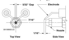
**Burner Air Adjustment:** The oil burner on this machine is preset for operation at altitudes below 500 feet. If operated at higher altitudes, it may be necessary to adjust the air band for a #1 or #2 smoke spot on the Bacharach scale.
