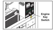
**STEP 3:** Turn engine key switch off.
