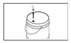
**STEP 1:** Remove detergent suction tube from container and insert into one gallon of fresh water. Open detergent valve, pull trigger on spray gun and siphon water for one minute.
