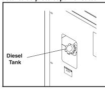
STEP 8: Fill diesel tank.
