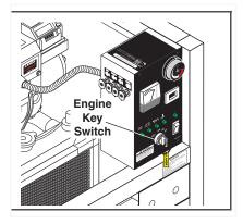
STEP 2: Read engine manual provided. The keyed ignition is located on the control panel. Simply turn key to first position. Glow plug light will illuminate. When light goes out, turn key to start (second) position.
