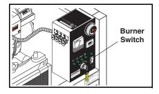
**STEP 2:** Turn burner switch off and continue spraying, allowing the water to cool to below 100°.
