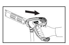
**STEP 5:** Squeeze trigger on spray gun to relieve remaining pressure.
