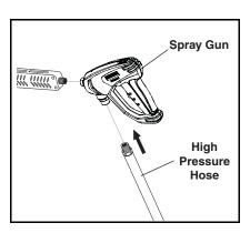
**STEP 4:** Attach the high pressure hose to the spray gun using teflon tape on hose threads.
