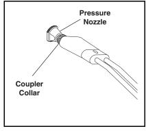
**STEP 6:** Release the coupler collar and push the nozzle until the collar clicks. Pull the nozzle to make sure it is seated properly.
