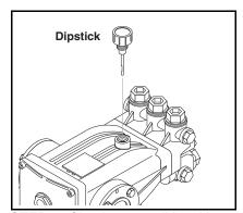
**STEP 7:** Check pump oil level by using supplied dip-stick. Use SAE 10W-40 non-foaming only.
