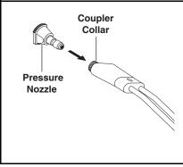
STEP 5: Before installing nozzle, turn on water supply and run machine allowing water to flush through the system until clear. Pull the springloaded collar of the wand coupler collar back to insert your choice of pressure nozzle. CAUTION: Never replace nozzles without engaging the safety latch on the spray gun trigger.
