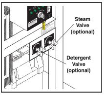
**STEP 5:** For steam, open the steam valve counterclockwise. This lowers the pressure and raises the temperature.
