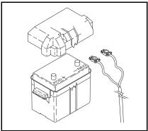
**STEP 9:** Install proper battery making sure that the red cable is attached to the positive terminal. Use a 12V group 24 style battery.
