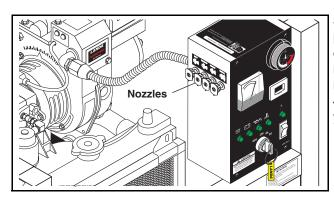
**STEP 6:** The four color-coded quick connect nozzles provide a wide array of spray widths from 0° to 45° and are easily accessible when placed in the convenient rubber nozzle holder, which is provided on the front of the machine. **NOTE:** For a more gentle rinse, select the white 40° or green 25° nozzle. To scour the surface, select the yellow 15° or red 0° nozzle.
