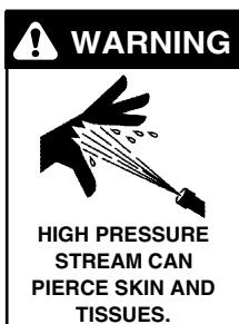
**WARNING: High pressure stream of fluid that this equipment can produce can pierce skin and its underlying tissues, leading to serious injury and possible amputation.**
