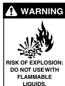
**WARNING: Do not use gasoline, crankcase drainings or oil containing gasoline, solvents or alcohol. Doing so will result in fire and/or explosion.**
