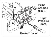
**STEP 8:** Connect the high pressure hose to the pump discharge nipple. Push coupler collar forward until secure.
