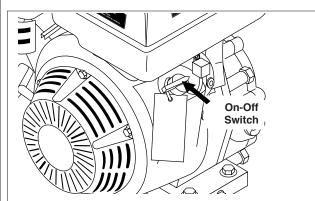
**STEP 8:** Turn the engine switch to "On" position. On Briggs engines, move the throttle lever to "Fast" position, shown on the engine as a rabbit.
