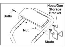
**STEP 3:** Attach the spray gun/ hose storage handle and bracket to handle. Tighten nuts.
