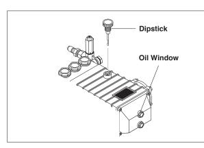
**STEP 2:** Remove shipping cap and install oil dipstick. Check pump oil level by using dipstick or observe oil level in oil window (if equipped). **Use 30 wt. (non detergent) oil.**
