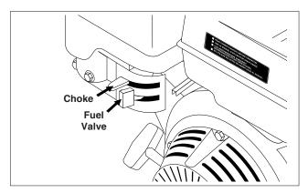
**STEP 5:** Rotate the fuel shut-off valve to the "On" position. Slide the fuel valve lever to the "ON" position. When the engine is not in use, leave the fuel valve in the "OFF" position.
