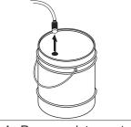
**STEP 1:** Remove detergent suction tube from container and insert into one gallon of fresh water. Slide nozzle forward for low pressure or to connect black detergent nozzle. Pull trigger on spray gun and siphon water for one minute.
