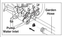
STEP 10: Check inlets filters, remove debris, then connect the garden hose to pump water inlet. *CAUTION: Do not run the pump without water or pump damage will result.*
