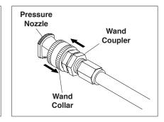
**STEP 6:** Pull the spring-loaded collar of the wand coupler back to insert your choice of pressure nozzle. Release the coupler collar and push the nozzle until the collar clicks. Pull the nozzle to make sure it is seated properly.
