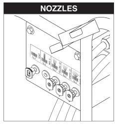
The four color-coded quick connect nozzles provide a wide array of spray widths from 15° to 40° and are easily accessible when placed in the convenient rubber nozzle holder, which is provided on the front of the machine.
