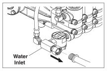
**STEP 4:** Disconnect the garden hose from the water inlet on the machine.
