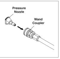
**STEP 2:** Pull the spring-loaded collar of the wand coupler back to insert your choice of pressure nozzle.
