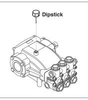
**STEP 4:** Remove shipping cap and install oil dipstick. Check pump oil level by using dipstick or observe oil level in oil window (if equipped). Use 20/40W non detergent oil.
