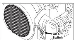
**STEP 2:** Turn engine switch to "OFF" position.
