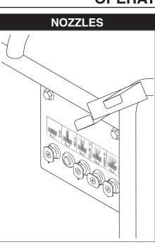
The four color-coded quick connect nozzles provide a wide array of spray widths from 15° to 40° and are easily accessible when placed in the convenient rubber nozzle holder, which is provided on the front of the machine.
