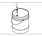
**STEP 1:** Remove detergent suction tube from container and insert into one gallon of fresh water. Slide nozzle forward for low pressure or to connect black detergent nozzle. Pull trigger on spray gun and siphon water for one minute.
