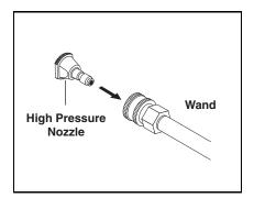
Note: Before installing pressure nozzle in wand coupler, run machine allowing water to flush through the system until clear.
