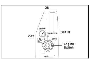
**STEP 8: (Electric Start Models)** Turn the key to the START position, and hold it there until the engine starts. If the engine fails to start within 5 seconds, release the key, and wait at least 10 seconds before operating the starter again.
