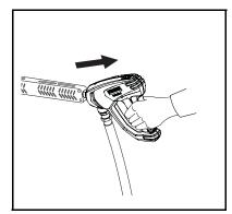
**STEP 4:** Before installing pressure nozzle, trigger spray gun to eliminate trapped pressure. Then run machine, allowing water to flush through the system until clear.
