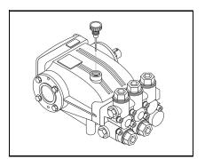
**STEP 3:** Remove shipping cap and install oil dipstick (Depending on type of shipping, dipstick may already be installed). Check pump oil level by using dipstick or observe oil level in oil window (if equipped). Use SAE 10W-40 weight oil, non-foaming oil.
