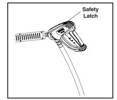
WARNING! Never replace nozzle without engaging the safety latch on the spray gun trigger.
