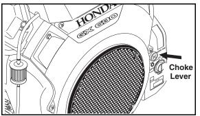
**STEP 5:** Pull the choke lever out to the "Choke" position (on a warm engine, leave the choke lever in the run position). Push the choke lever to the "Closed" position. To restart a warm engine, leave the choke lever in the "Open" position.
