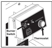
**STEP 9:** Turn the burner switch "ON". Turn thermostat dial to the 210° mark.
