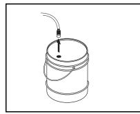
**STEP 1:** Remove detergent suction tube from container and insert into one gallon of fresh water. Open detergent metering valve. Pull trigger on spray gun and siphon water for one minute. Close detergent valve. Turn burner switch off and continue spraying, allowing the water to cool to below 100°F.
