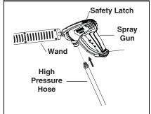
**STEP 1:** Attach wand and hose to the spray gun using teflon tape on threads to prevent leakage. *CAUTION: Never replace nozzles without engaging the safety latch on the spray gun trigger.*
