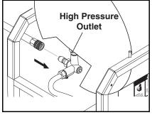
**STEP 7:** Disconnect the high pressure hose from high pressure outlet.
