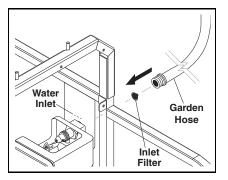
**STEP 5:** Check inlet filters, remove debris, then connect the water supply hose to the float tank inlet swivel connector and turn on water supply.
