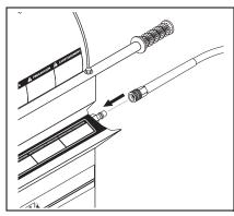
**STEP 1:** Connect the high pressure hose quick coupler from attached pressure washer to discharge nipple by sliding the quick coupler collar back and inserting quick coupler on coupler nipple and pushing the quick coupler collar forward to secure it.
