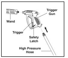
**STEP 3:** Attach variable pressure control wand to spray gun using teflon tape on threads to prevent leakage. Position safety latch to prevent trigger from being pulled.
