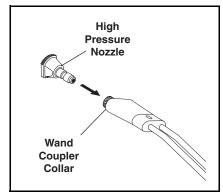
**STEP 4:** Pull the spring-loaded collar of the wand coupler collar back to insert your choice of pressure nozzle.
