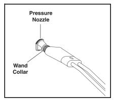
**STEP 5:** Release the coupler collar and push the nozzle until the collar clicks. Pull the nozzle to make sure it is seated properly.
