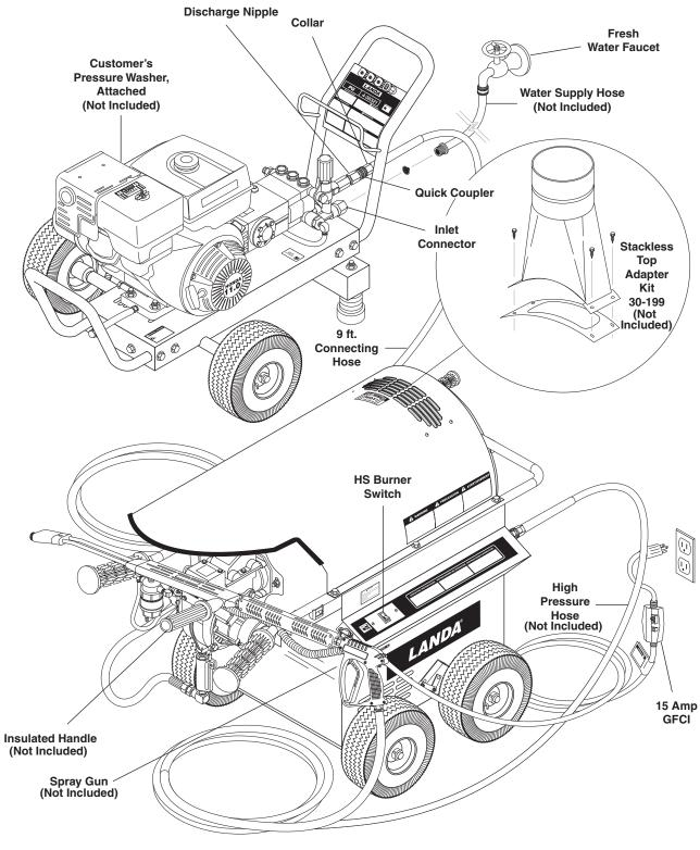
NOTE: The water in this machine is hot. The wand and spray gun must be insulated
