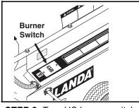
**STEP 2:** Turn HS burner switch off and continue spraying water, allowing the water to cool.
