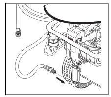
**STEP 2:** Connect high pressure hose from the attached pressure washer (not included) to the hot water discharge nipple by sliding quick coupler collar back. Insert quick coupler onto discharge nipple and secure by pushing quick coupler collar forward. (See Component Identification)
