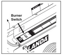
**STEP 3:** For hot water washing, turn the HS burner switch to the ON position. (The burner will light automatically.)
