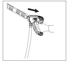
**STEP 3:** Open spray gun to relieve remaining pressure and remove water supply hose.
