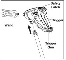
**STEP 5:** Attach variable pressure control wand to spray gun using teflon tape on threads to prevent leakage. Position safety latch to prevent trigger from being pulled.
