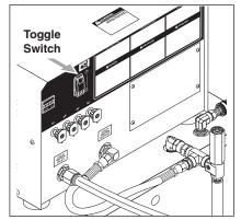
**STEP 3:** Place toggle switch in the ON position and then pull the trigger on the spray gun to activate a pressure switch which will then start the machine. The ON position is for auto shut down.
