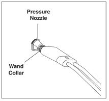
**STEP 7:** Release the coupler collar and push the nozzle until the collar clicks. Pull the nozzle to make sure it is seated properly.
