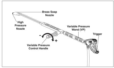
**STEP 4:** Turn the variable pressure control handle clockwise to increase pressure.
