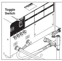
**STEP 1:** Rinse all lines (and injector) with clean water, to remove any soap residue then turn toggle switch off.
