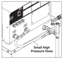
**STEP 2:** Place the pump package on top of the heat exchange and attach the small high pressure hose to the fittings as shown.
