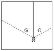
**STEP 1:** Place machine in a convenient location providing ample support, drainage and room for maintenance. Remove pallet bolts and remove pallet, then re-install bolts to level machine by adjusting (machine must be level).
