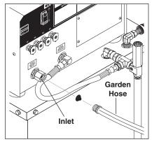
**STEP 2:** Connect water supply hose (garden hose) to inlet connector. Do not allow acid or abrasives to be pumped through system. Turn on water.
