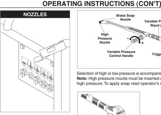
**Brass Soap** Nozzle Variable Pressure Wand (VP) Hìgh Pressure Nozzle Variable Pressure Trigger **Control Handle**
