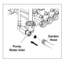
**STEP 7:** Check inlet filters, remove debris, then connect garden hose to pump water inlet. *CAUTION: Do not run the pump without water or pump damage will result.*
