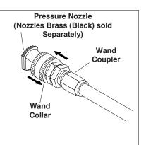
**STEP 3:** Release the coupler collar and push the nozzle until the collar clicks. Pull the nozzle to make sure it is seated properly.
