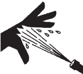
RISK OF INJECTION OR SEVERE INJURY TO PERSONS. KEEP CLEAR OF NOZZLE.
