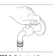
**STEP 3:** Before installing nozzle, turn on water supply and run machine allowing water to flush through the system until clear.
