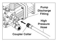
**STEP 4:** Connect the high pressure hose to the pump discharge fitting. Push coupler collar forward until secure.
