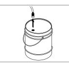
**STEP 1:** Remove detergent suction tube from container and insert into one gallon of fresh water. Slide nozzle forward for low pressure or to connect black detergent nozzle. Pull trigger on spray gun and siphon water for one minute.
