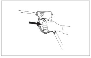
**STEP 4:** Trigger the spray gun to eliminate trapped air then wait for a steady flow of water to emerge from the spray nozzle.
