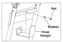
**STEP 3:** Use the nut and washer to attach the hose hanger.
