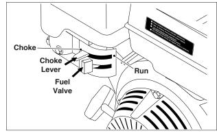
**STEP 7:** Move the choke lever to the "Choke" position (on a warm engine, leave the choke lever in the run position).
