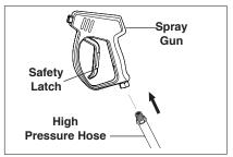
**STEP 4:** Attach the high pressure hose to the spray gun using teflon tape on hose threads.
