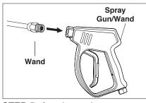
**STEP 5:** Attach wand to spray gun using teflon tape on wand threads.
