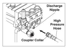
**STEP 8:** Connect the high pressure hose to the discharge nipple. Push coupler collar forward until secure.
