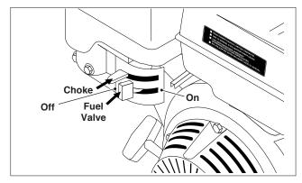
**STEP 6:** Slide the fuel valve lever to the "ON" position. When the engine is not in use, leave the fuel valve in the "OFF" position.
