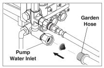
STEP 10: Check inlets filters, remove debris, then connect the garden hose to pump water inlet. CAUTION: Do not run the pump without water or pump damage will result.
