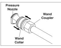
**STEP 7:** Release the coupler collar and push the nozzle until the collar clicks. Pull the nozzle to make sure it is seated properly.
