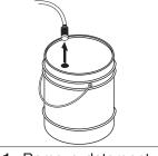
**STEP 1:** Remove detergent suction tube from container and insert into one gallon of fresh water. Slide nozzle forward for low pressure or to connect black detergent nozzle. Pull trigger on spray gun and siphon water for one minute.
