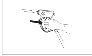
**STEP 4:** Trigger the spray gun to eliminate trapped air then wait for a steady flow of water to emerge from the spray nozzle.
