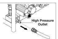
STEP 6: Disconnect the high pressure hose from high pressure outlet.
