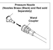
**STEP 2:** Pull the spring-loaded collar of the wand coupler back to insert your choice of pressure nozzle.
