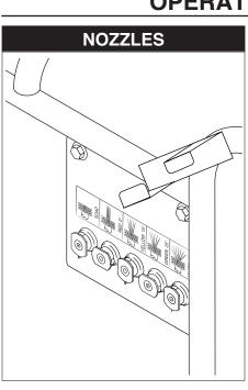
The five color-coded quick connect nozzles provide a wide array of spray widths from 0° to 40° and are easily accessible when placed in the convenient rubber nozzle holder, which is provided on the front of the machine.
