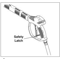
WARNING! Never replace nozzles without engaging the safety latch on the spray gun trigger.
