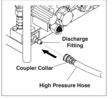
**STEP 5:** Connect the high pressure hose to the pump discharge fitting. Push coupler collar forward until secure.
