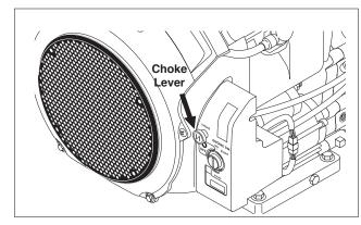
**STEP 5:** Pull the choke lever out to the "Choke" position (on a warm engine, leave the choke lever in, in the run position). Push the choke lever to the "Closed" position. To restart a warm engine, leave the choke lever in the "Open" position.
