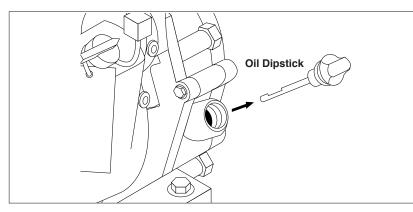
**STEP 1:** Check engine oil level. Oil level should be level with the bottom of the oil filler neck. Be sure the machine is level when checking the oil level. (Refer to the engine's operating manual included with machine.) We recommend that the oil be changed after the first 5 hours of use, then once every 50 hours. **Note:** Improper oil levels will cause low oil sensor to shut off engine. **IMPORTANT! Do not run engine with high or low oil levels as this will cause engine damage.**
