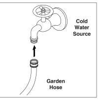
**STEP 4:** Connect garden hose to the cold water source and turn water on completely. Never use hot water.
