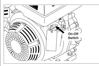
**STEP 8:** Turn the engine switch to "On" position. On Vanguard engines, move the throttle lever to "Fast" position, shown on the engine as a rabbit.
