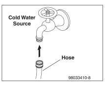
**STEP 6:** Connect one end of hose to the cold water source.
