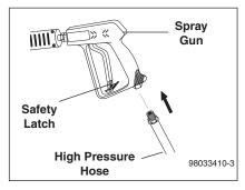
**STEP 1:** Attach the high pressure hose to the spray gun using teflon tape on hose threads.
