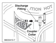
**STEP 5:** Connect the high pressure hose to the pump discharge fitting. Push coupler collar forward until secure.
