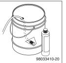
**STEP 1:** Use detergent designed specifically for pressure washers. Household detergents could damage the pump. Prepare detergent solution as required by the manufacturer. Fill a container with pressure washer detergent. Place the filter end of detergent suction
