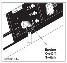
**STEP 4:** Read engine operators manual before starting. Turn the key to GL (Glow Plug) and wait for light to go out. Turn the engine switch to ST (Start) position.
