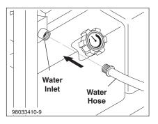
STEP 7: Connect the other end of the water hose to pump water inlet. Inspect inlets. *CAUTION: Do not run the pump without water or pump damage will result.*
