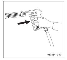
**STEP 3:** Before installing nozzle, trigger the spray gun to eliminate trapped air then wait for a steady flow of water to emerge from the wand coupler when engine starts. Run machine allowing water to flush through the system until clear.
