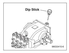
**STEP 4:** Remove shipping cap and install oil dipstick. Check pump oil level by using dipstick or observe oil level in oil window (if equipped). Use 10W-40 non detergent pump oil.
