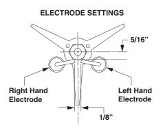
Periodically Check Wiring Connections. If Necessary to adjust electrodes, use diagram.
