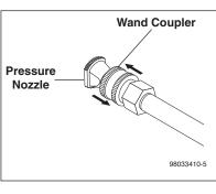
**STEP 3:** Release the coupler collar and push the nozzle in until the collar clicks. Pull the nozzle to make sure it is seated properly.
