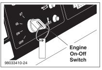
**STEP 2:** Turn key to stop position. Engine shuts down by way of solenoid.
