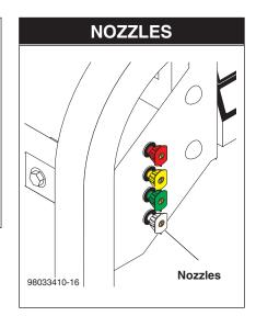
The quick connect nozzles provide a wide array of spray widths from  $0^{\circ}$  to  $40^{\circ}$  and are easily accessible when placed in the convenient rubber nozzle holder, which is provided on the front of the machine.
