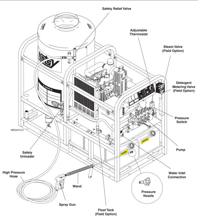
**Pump** — Develops high pressure by pumping water volume through nozzle.
