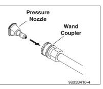
**STEP 2:** Pull the spring-loaded collar of the wand coupler back to insert your choice of pressure nozzle.
