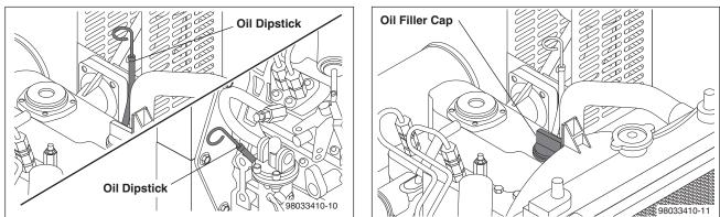
**STEP 1:** Check engine oil level. Oil level should be between the lines on the dipstick. (Refer to the engine's operating manual included with machine.) We recommend that the oil be changed after the first 5 hours of use, then once every 50 hours. **NOTE:** Improper oil levels will cause low oil sensor to shut off engine. *IMPORTANT! Do not run engine with high or low oil levels as this will cause engine damage.*
