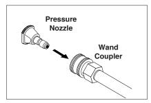
**STEP 3:** Pull spring-loaded collar of the wand coupler back to insert your choice of pressure nozzle.
