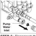
**STEP 5:** Disconnect the garden hose from the water inlet on the machine.
