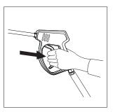
**STEP 4:** Press trigger to release water pressure.
