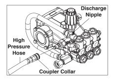
**STEP 5:** Connect the high pressure hose to the discharge nipple. Push coupler collar forward until secure.
