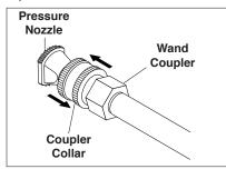
**STEP 4:** Release the coupler collar and push the nozzle until the collar clicks. Pull the nozzle to make sure it is seated properly.
