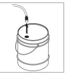
**STEP 1:** Remove detergent suction tube from container and insert into one gallon of fresh water. Slide nozzle forward for low pressure or use black detergent nozzle. Pull trigger on spray gun and siphon fresh clean water for one minute.
