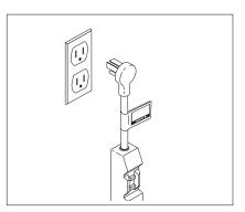
**STEP 3:** Connect to appropriate power supply. Push reset button on GFCI.
