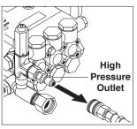
**STEP 6:** Disconnect the high pressure hose from the discharge nipple.
