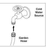
**STEP 1:** Connect garden hose to the cold water source and turn water on completely. Never use hot water.
