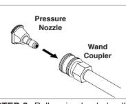
**STEP 3:** Pull spring-loaded collar of the wand coupler back to insert your choice of pressure nozzle.
