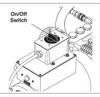
**STEP 4:** Turn machine on by turning switch at top of motor.
