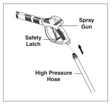
**STEP 1:** Attach the high pressure hose to the spray gun using teflon tape on hose threads.
