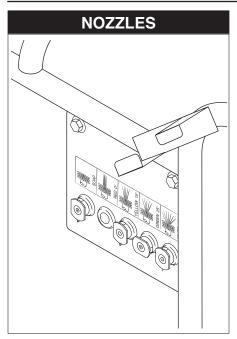
The four color-coded quick connect nozzles provide a wide array of spray widths from 15° to 40° and are easily accessible when placed in the convenient rubber nozzle holder, which is provided on the front of the machine.
