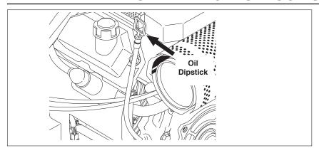
STEP 1: Check engine oil level. Oil level should be level with the bottom of the oil filler neck. Be sure the machine is level when checking the oil level. (Refer to the engine's operating manual included with machine.) We recommend that the oil be changed after the first 5 hours of use, then once every 50 hours. Note: Improper oil levels will cause low oil sensor to shut off engine. IMPORTANT! Do not run engine with high or low oil levels as this will cause engine damage.
