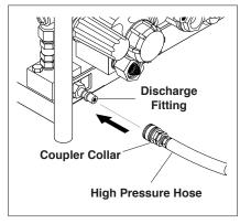
**STEP 5:** Connect the high pressure hose to the pump discharge fitting. Push coupler collar forward until secure.
