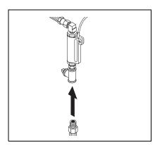
**STEP 2:** Connect high pressure hose from pressure washer (not included) to burner module.
