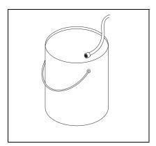
**STEP 1:** To clean detergent from hose and wand, insert end of detergent hose in clean bucket of water and run for a few minutes until steady stream of clean water is evident.
