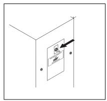
**STEP 2:** Turn burner switch off and continue spraying, allowing the water to cool to below 100°F.
