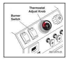
**STEP 4:** For hot water, turn the thermostat knob to 210° then push the burner switch to ON when a steady stream of water flows out of the spray gun. Burner will now light automatically. **NOTE:** Do not start machine with burner switch on.
