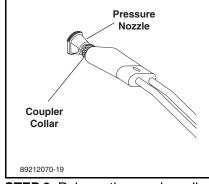
**STEP 6:** Release the coupler collar and push the nozzle until the collar clicks. Pull the nozzle to make sure it is seated properly.
