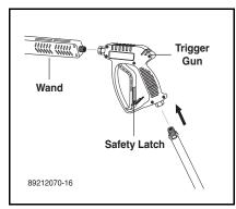
**STEP 3:** Attach variable pressure control wand to spray gun using teflon tape on threads to prevent leakage.
