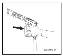
**STEP 3:** With the spray nozzle pointed away from you or anybody else, press the trigger on the spray gun to obtain pressurized cold water spray.
