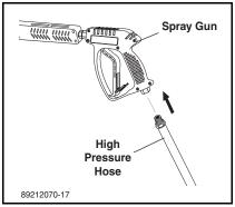
**STEP 4:** Attach the high pressure hose to the spray gun using teflon tape on hose threads.
