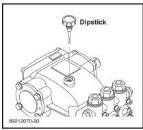
**STEP 7:** Check oil level by using supplied dip-stick. Use SAE 10W-40 non-foaming only.
