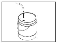
**STEP 1:** Remove detergent suction tube from container and insert into one (1) gallon of fresh water. Pull trigger on spray gun and siphon water for one minute
