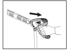
**STEP 3:** After water has cooled, turn the pump switch off.
