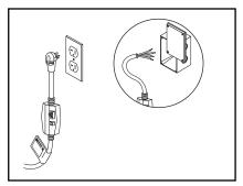
STEP 1: Machines must be stored indoors when not in use. Location of machine is important. Avoid installing near combustible material or in poorly ventilated areas. Electrical connection to machine should be the proper voltage, phase and amperage. See specifications for particular model. Plug the power cord into a grounded receptacle.
