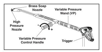
**STEP 5:** Selection of high or low pressure is accompanied by turning the handle. **Note:** High pressure nozzle must be inserted at end of wand to obtain high pressure. To apply soap, see Detergent and General Cleaning Techniques section.
