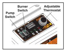
**STEP 4:** Press the pump switch "ON" and then pull the trigger on the spray gun to activate pressure switch which starts machine (For auto start machines only).
