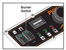
**STEP 2:** Push burner switch off and open trigger on spray gun, allowing water to flow, which will cool down the heating coil.
