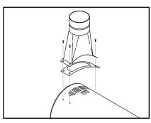
STEP 4: Adding exhaust vent pipe to your oil fired burner is not recommended because it restricts air flow. This causes carbon build-up, which affects the operation and increases maintenance on the coil. If a stack must be used, refrain from using 90° bends. If the pipe can not go straight up then use only 45° bends and go to the next larger size pipe. The overall pipe length must not exceed 6 feet in length. Air adjustments will be required after installation.
