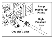
**STEP 4:** Connect the high pressure hose to the pump discharge fitting. Push coupler collar forward until secure.
