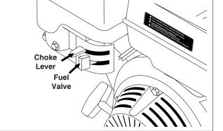
**STEP 6:** Rotate the fuel shut-off valve to the "On" position (fully counterclockwise on Briggs engines). Slide the fuel valve lever to the "ON" position (Honda engines). When the engine is not in use, leave the fuel valve in the "OFF" position.
