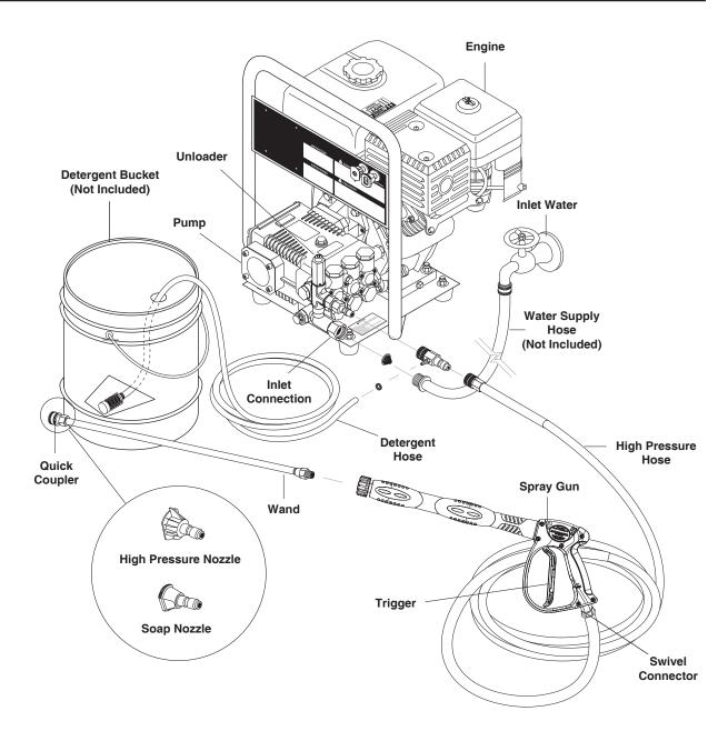
**Detergent Injector** - Allows you to siphon and mix detergents.
