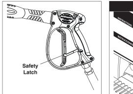
WARNING! Never replace nozzles without engaging the safety latch on the spray gun trigger. NOZZLES
