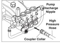
**STEP 8:** Connect the high pressure hose to the pump discharge nipple. Push coupler collar forward until secure.
