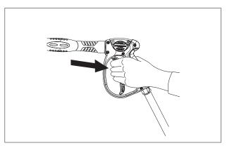
STEP 4: Trigger the spray gun to eliminate trapped air then wait for a steady flow of water to emerge from the spray nozzle.
