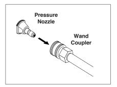
**STEP 6:** Pull the spring-loaded collar of the wand coupler back to insert your choice of pressure nozzle.
