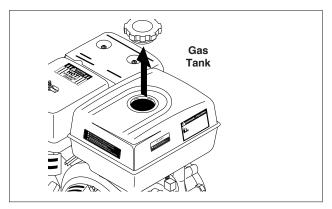
STEP 3: Fill gas tank with unleaded gasoline. Do not use leaded gasoline.
