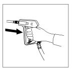
**STEP 4:** Press trigger to release water pressure.
