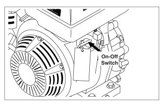
**STEP 8:** Turn the engine switch to "On" position. On Briggs engines, move the throttle lever to "Fast" position, shown on engine as a rabbit.
