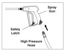
**STEP 4:** Attach the high pressure hose to the spray gun using teflon tape on hose threads.
