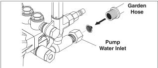
STEP 9: Connect the garden hose to pump water inlet. Inspect inlets. *CAUTION: Do not run the pump without water or pump damage will result.*
