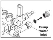
STEP 5: Disconnect the garden hose from the water inlet on the machine.
