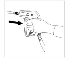
**STEP 5:** Trigger the spray gun to eliminate trapped air then wait for a steady flow of water to emerge from the spray nozzle.
