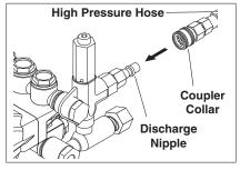
**STEP 7:** Connect high pressure hose to pumps discharge nipple. Push coupler collar forward until secure.
