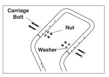
**STEP 2:** Insert the carriage bolt through the holes from the outside of the unit and attach a nut from the inside of the machine. Tighten nuts.
