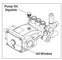
**STEP 2:** Remove shipping cap and install oil dipstick. Check pump oil level by using dipstick or observe oil level in oil window (if equipped). Use 30 wt. (non detergent) oil.
